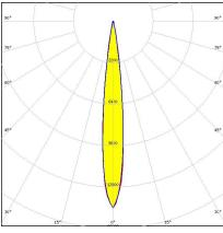
Dimensions: 40.0 mm x 40.0 mm Height: 10.70 mm ~20° medium beam with 7 optics
