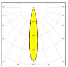
Dimensions: 40.0 mm x 40.0 mm Height: 10.70 mm ~15° spot beam with 7 optics
