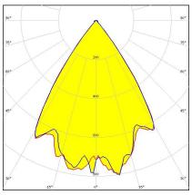
Dimensions: 40.0 mm x 40.0 mm Height: 12.15 mm ~65° wide beam with 7 optics
