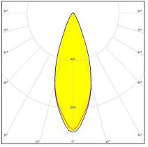
Dimensions: 40.0 mm x 40.0 mm Height: 10.70 mm ~30° wide beam with 6 optics
