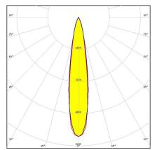
Dimensions: 40.0 mm x 40.0 mm Height: 10.70 mm ~15° spot beam with 6 optics
