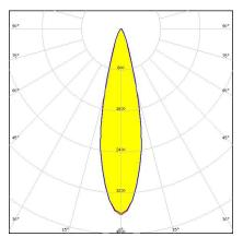
Dimensions: 40.0 mm x 40.0 mm Height: 10.70 mm ~20° medium beam with 6 optics
