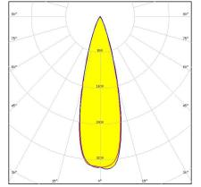
Dimensions: 40.0 mm x 40.0 mm Height: 10.70 mm ~25° medium beam with 7 optics
