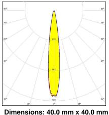
Dimensions: 40.0 mm x 40.0 mm Height: 10.70 mm ~15° spot beam with 7 optics
