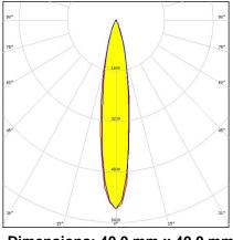
Dimensions: 40.0 mm x 40.0 mm Height: 10.70 mm ~15° spot beam with 5 optics
