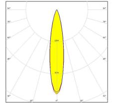
Dimensions: 40.0 mm x 40.0 mm Height: 10.70 mm ~20° medium beam with 7 optics
