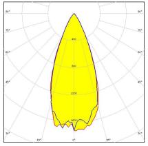
Dimensions: 40.0 mm x 40.0 mm Height: 10.70 mm ~30° wide beam with 7 optics
