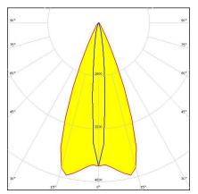
Dimensions: 26.0 mm x 26.0 mm Height: 14.97 mm ~45° x 10° oval beam. 14.97 mm high lens.
