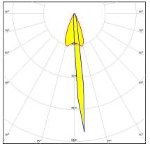
Dimensions: 26.0 mm x 26.0 mm Height: 14.95 mm ~45° x 10° oval beam for wall washing. 14.95 mm high lens.
