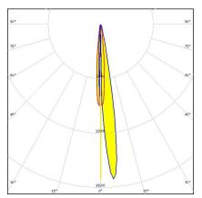
Dimensions: 26.0 mm x 26.0 mm Height: 14.83 mm ~8° beam for wall-washing. 14.83 mm high lens.
