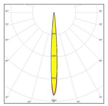
Dimensions: 26.0 mm x 26.0 mm Height: 14.74 mm ~8° spot beam. 14.74 mm high lens.
