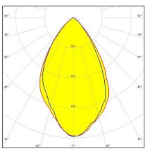
Dimensions: 26.0 mm x 26.0 mm Height: 13.43 mm ~60° wide beam. 13.43 mm high lens. Modified version to fit CREE
