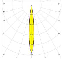
Dimensions: 26.0 mm x 26.0 mm Height: 14.82 mm ~11° smooth spot beam. 14.82 mm high lens.
