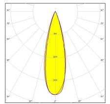
Dimensions: 26.0 mm x 26.0 mm Height: 14.88 mm ~30° medium beam. 14.88 mm high lens.
