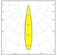
Dimensions: 26.0 mm x 26.0 mm Height: 14.85 mm ~20° medium beam. 14.85 mm high lens.
