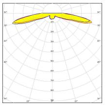
Dimensions: 9.9 mm x 9.9 mm Height: 5.70 mm ~170° side emitter
