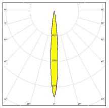
Dimensions: 21.6 mm x 21.6 mm Height: 14.30 mm ~9.6° spot beam optimized for Osram
