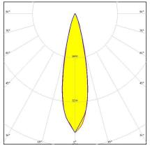
Dimensions: 21.6 mm x 21.6 mm Height: 14.04 mm ~14° diffused spot beam optimized for
