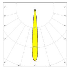
Dimensions: 21.6 mm x 21.6 mm Height: 14.70 mm ~8.5° spot beam optimized for CREE XP-E. 14.7 mm high assembly with
