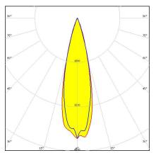
Dimensions: 21.8 mm x 21.8 mm Height: 14.70 mm ~20° medium beam with light, black holder. Assembly with installation tape.
