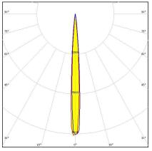
Dimensions: 21.6 mm x 21.6 mm Height: 14.70 mm ~9.6° spot beam optimized for CREE
