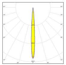
Dimensions: 21.6 mm x 21.6 mm Height: 14.70 mm ~9.6° spot beam optimized for CREE XP-E. 14.7 mm high assembly with installation tape.
