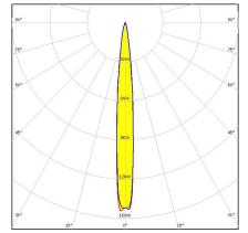
Dimensions: 21.6 mm x 21.6 mm Height: 14.70 mm ~8.5° spot beam optimized for CREE
