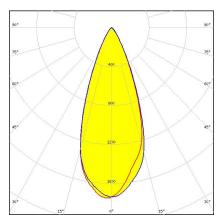
**Dimensions: 21.8 mm x 21.8 mm Height: 14.70 mm** ~40° wide beam with light, black holder. Assembly with location pins and installation tape.
