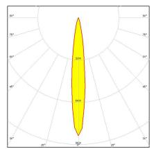
Dimensions: 21.6 mm x 21.6 mm Height: 14.70 mm ~14° diffused spot beam optimized for CREE XP-E. 14.7 mm high assembly with installation tape.
