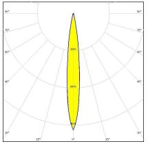
Dimensions: 21.6 mm x 21.6 mm Height: 16.50 mm ~9.6° spot beam optimized for CREE XR-E. 16.5 mm high assembly with installation tape.
