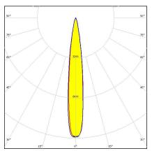
**Dimensions: 21.8 mm x 21.8 mm Height: 14.70 mm** ~8.5° spot beam with light, black holder. Assembly with installation tape.
