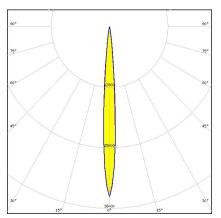
**Dimensions: 21.8 mm x 21.8 mm Height: 14.70 mm** ~8.5° spot beam with light, black holder. Assembly with location pins and installation tape.
