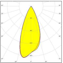
Dimensions: 21.6 mm x 21.6 mm Height: 14.70 mm ~40° wide beam optimized for CREE
