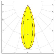
Dimensions: 21.6 mm x 21.6 mm Height: 13.50 mm ~35° x 25° rectangular beam optimized for Nichia NS6x83. 13.3 mm high assembly with installation tape.
