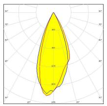
Dimensions: 21.6 mm x 21.6 mm Height: 14.70 mm ~40° wide beam optimized for CREE XP-E. 14.7 mm high assembly with
