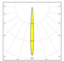
Dimensions: 21.6 mm x 21.6 mm Height: 14.70 mm ~9.6° spot beam optimized for CREE XP-E. 14.7 mm high assembly.
