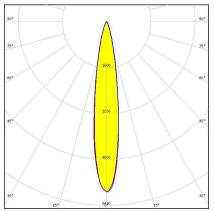
**Dimensions: 21.8 mm x 21.8 mm Height: 14.70 mm** ~14° diffused spot beam with light, black holder. Assembly with installation tape.
