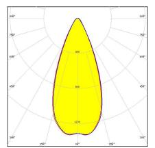
Dimensions: 52.1 mm x 52.1 mm Height: 16.98 mm ~45° wide beam with holder C compatible with LEDiL HEKLA
