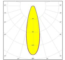
Dimensions: 69.9 mm x 69.9 mm Height: 17.20 mm ~25° spot beam with holder A compatible with 3rd party connectors from TE, Bender+Wirth and IDEAL
