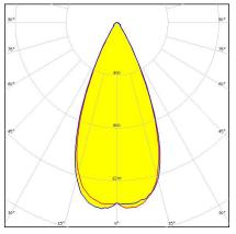
Dimensions: 69.9 mm x 69.9 mm Height: 14.00 mm ~45° wide beam with holder A compatible with 3rd party connectors
