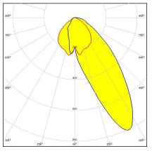
Dimensions: 53.9 mm x 53.9 mm Height: 16.00 mm Asymmetric wall washing beam ideal
