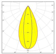
Dimensions: 53.9 mm x 53.9 mm Height: 20.50 mm ~50° + 30° oval beam with holder C compatible with LEDiL HEKLA
