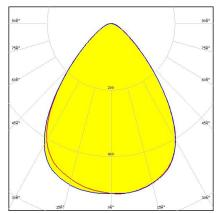
Dimensions: 53.9 mm x 53.9 mm Height: 17.00 mm ~90° wide beam with holder C compatible with LEDiL HEKLA
