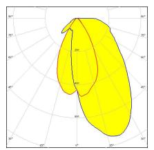
Dimensions: 69.9 mm x 69.9 mm Height: 22.30 mm Asymmetric beam for wall washing with holder B compatible with 3rd party connectors from BJB, IDEAL and Stucchi
