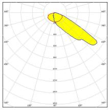
**Dimensions: 25.0 mm x 25.0 mm Height: 12.40 mm** Forward throw beam for area lighting.
