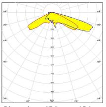
**Dimensions: 25.0 mm x 25.0 mm Height: 11.70 mm** Wide IESNA Type IV beam with forward-throw beam for wide area lighting like car parks.
