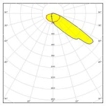
**Dimensions: 25.0 mm x 25.0 mm Height: 12.60 mm** Forward throw beam for area lighting. Assembly with installation tape.
