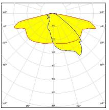
Dimensions: 25.0 mm x 25.0 mm Height: 8.20 mm IESNA Type III (medium) beam with
