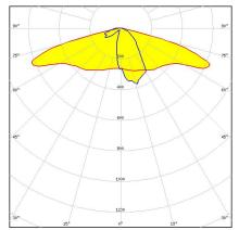
Dimensions: 25.0 mm x 25.0 mm Height: 8.60 mm IESNA Type II (medium) beam,
