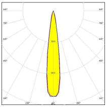
Dimensions: 16.0 mm x 16.0 mm Height: 9.50 mm ~14° spot beam. Assembly with holder,
