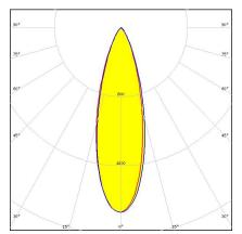
Dimensions: 16.1 mm x 16.1 mm Height: 11.00 mm ~30° medium beam optimized for Nichia NS6x83. Assembly with holder and installation tape.
