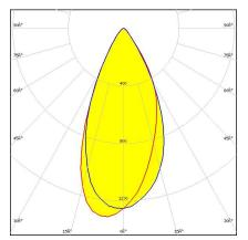
Dimensions: 16.1 mm x 16.1 mm Height: 9.30 mm ~45° wide beam optimized for Nichia NCSxx19. Assembly with holder, installation tape and location pins.
