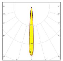
Dimensions: 16.1 mm x 16.1 mm Height: 9.50 mm ~14° spot beam optimized for Osram Oslon SSL80. Assembly with holder.
