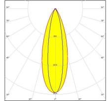
Dimensions: 16.1 mm x 16.1 mm Height: 11.00 mm ~35° + 15° oval beam optimized for
