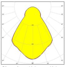
**Dimensions: 16.1 mm x 16.1 mm Height: 10.10 mm** Mini reflector with ~60° wide beam and clip installation
