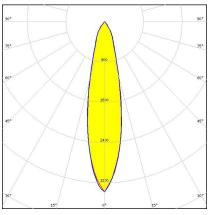
Dimensions: 69.6 mm x 69.6 mm Height: 39.90 mm ~24° medium beam
