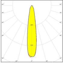
Dimensions: 69.6 mm x 69.6 mm Height: 39.90 mm ~15° spot beam
