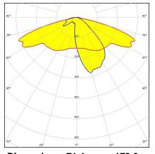
Dimensions: 71.4 mm x 173.0 mm Height: 9.17 mm IESNA Type II (medium) beam applicable for European P-class standard pedestrian lighting and M-class roads
