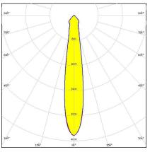
Dimensions: 49.8 mm x 49.8 mm Height: 17.98 mm ~15° spot beam
