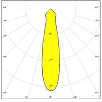
Dimensions: 49.8 mm x 49.8 mm Height: 17.98 mm ~24° medium beam
