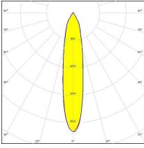
Dimensions: 49.9 mm x 49.9 mm Height: 25.00 mm ~24° medium beam
