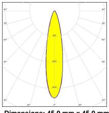
Dimensions: 45.0 mm x 45.0 mm Height: 11.90 mm Infinitely adjustable beam from 20 to 50 degrees.
