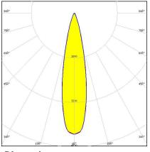
Dimensions: mm x mm Height: mm ~18° spot beam
