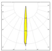
Dimensions: 119.5 mm x 119.5 mm Height: 74.50 mm ~10° spot beam compatible with BJB and B+W connectors
