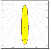
Dimensions: 119.5 mm x 119.5 mm Height: 74.50 mm ~30° medium beam compatible with BJB and B+W connectors
