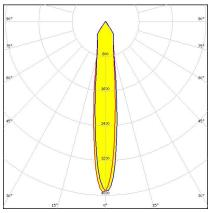
Dimensions: 119.5 mm x 119.5 mm Height: 74.27 mm ~30° medium beam
