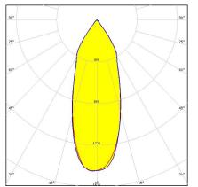
Dimensions: 119.5 mm x 119.5 mm Height: 74.50 mm ~45° wide beam compatible with BJB and B+W connectors
