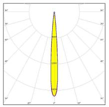
Dimensions: 119.5 mm x 119.5 mm Height: 74.27 mm ~10° spot beam
