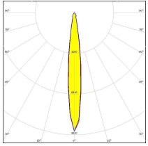
Dimensions: 70.0 mm x 70.0 mm Height: 41.70 mm ~15° spot beam
