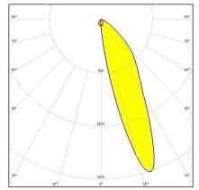
Dimensions: 21.5 mm x 21.5 mm Height: 16.10 mm Asymmetric beam for billboards. Assembly with holder.
