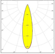
Dimensions: 279.5 mm x 12.5 mm Height: 9.77 mm ~30° medium beam
