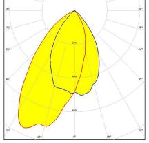
Dimensions: 139.5 mm x 9.4 mm Height: 5.25 mm Asymmetric beam for wall-washing
