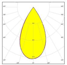
Dimensions: 1140.0 mm x 40.0 mm Height: 20.20 mm ~50° wide beam. Variant with 7X1 lenses.
