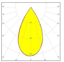
Dimensions: 1140.0 mm x 40.0 mm Height: 20.20 mm ~50° wide beam. Variant with diffused 7X1 lenses.
