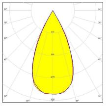
Dimensions: 1140.0 mm x 40.0 mm Height: 20.20 mm ~50° wide beam with tighter cutoff. Variant with 7X1 lenses.
