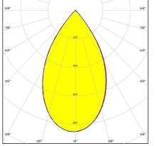
Dimensions: 1140.0 mm x 40.0 mm Height: 20.20 mm ~50° wide beam. Variant with diffused 4X1 lenses.
