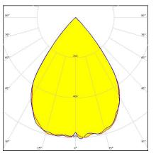
Dimensions: 200.0 mm x 200.0 mm Height: 20.40 mm ~80° wide beam. Variant with diffused lenses.
