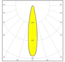
Dimensions: 32.0 mm x 32.0 mm Height: 20.00 mm ~28° wide beam. Assembly with black holder.
