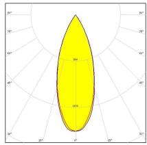
Dimensions: 32.0 mm x 32.0 mm Height: 20.00 mm ~38° wide beam. Assembly with black holder.
