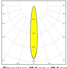
Dimensions: 29.6 mm x 29.6 mm Height: 17.20 mm ~15° spot beam
