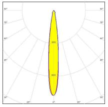
Dimensions: 32.0 mm x 32.0 mm Height: 20.00 mm ~15° spot beam. Assembly with black holder.
