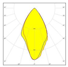
Dimensions: 26.0 mm x 26.0 mm Height: 13.43 mm ~60° wide beam. 13.43 mm high lens.
