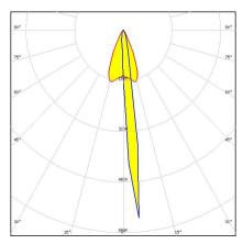
Dimensions: 26.0 mm x 26.0 mm Height: 14.95 mm ~45° x 10° oval beam for wall
