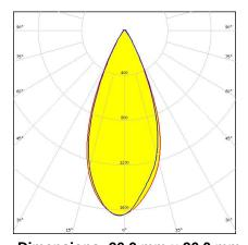
Dimensions: 26.0 mm x 26.0 mm Height: 14.74 mm ~45° wide beam. 14.74 mm high
