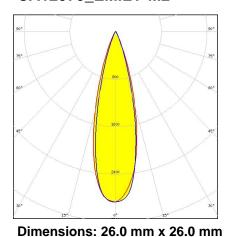
Height: 14.88 mm ~30° medium beam. 14.88 mm high lens.
