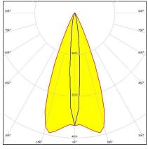
Dimensions: 26.0 mm x 26.0 mm Height: 14.97 mm ~45° x 10° oval beam. 14.97 mm
