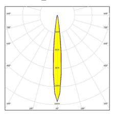
Dimensions: 26.0 mm x 26.0 mm Height: 14.82 mm ~11° smooth spot beam. 14.82 mm
