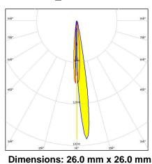
Height: 14.83 mm ~8° beam for wall-washing. 14.83 mm high lens.
