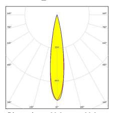
Dimensions: 26.0 mm x 26.0 mm Height: 14.85 mm ~20° medium beam. 14.85 mm high
