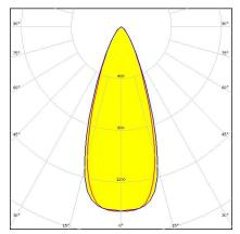
Dimensions: 26.0 mm x 26.0 mm Height: 14.74 mm ~40° wide beam 14.74 mm high
