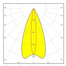
Dimensions: 26.0 mm x 26.0 mm Height: 14.96 mm ~45° x 10° oval beam. 14.96 mm
