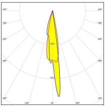
Dimensions: 32.8 mm x 32.8 mm Height: 17.41 mm 10+20° asymmetric beam
