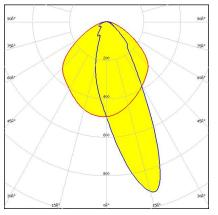
Dimensions: 19.5 mm x 286.0 mm Height: 7.13 mm Asymmetric beam for wall-washing
