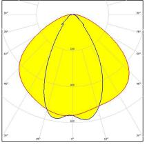
**Dimensions: 19.5 mm x 286.0 mm Height: 7.55 mm** ~60° + 110° medium beam
