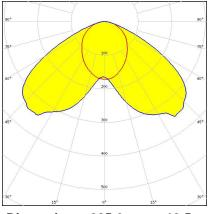
Dimensions: 285.6 mm x 19.5 mm Height: 6.91 mm Asymmetric beam for uplighting
