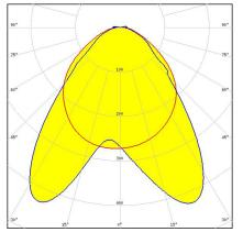
Dimensions: 19.5 mm x 286.0 mm Height: 6.40 mm Double asymmetric beam for aisle and shelf lighting
