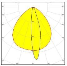
Dimensions: 21.7 mm x 286.0 mm Height: 11.04 mm Asymmetric oval beam for wall grazing
