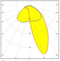
Dimensions: 286.0 mm x 61.0 mm Height: 11.38 mm Single-sided asymmetric oval beam for aisle lighting
