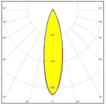
Dimensions: 286.0 mm x 61.0 mm Height: 8.50 mm ~30° medium beam
