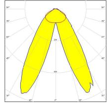
Dimensions: 286.0 mm x 61.0 mm Height: 11.00 mm Double asymmetric beam for aisle and
