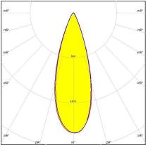
Dimensions: 45.0 mm x 45.0 mm Height: 28.84 mm ~35° wide beam with holder
