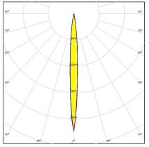
Dimensions: 45.0 mm x 45.0 mm Height: 29.10 mm ~9° spot beam with holder and installation tape
