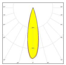
Dimensions: 45.0 mm x 45.0 mm Height: 29.24 mm ~25° medium beam with holder and installation tape
