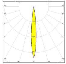
Dimensions: 45.0 mm x 45.0 mm Height: 29.20 mm ~11° smooth spot beam with holder
