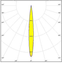
Dimensions: 45.0 mm x 45.0 mm Height: 28.90 mm ~9° spot beam with holder
