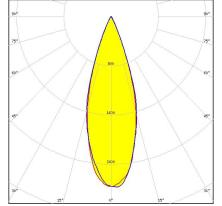
Dimensions: 45.0 mm x 45.0 mm Height: 29.24 mm ~35° wide beam with holder and installation tape
