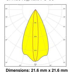
**Height: 11.70 mm** ~13° x 45° oval beam optimized for Luxeon Rebel. Variant with beam direction rotated 90°.
