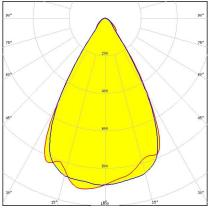
**Dimensions: 172.0 mm x 71.0 mm Height: 8.20 mm** ~60° wide beam. Variant made from PC.
