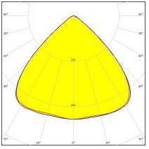
Dimensions: 172.0 mm x 71.0 mm Height: 8.20 mm ~90° wide beam. Variant made from PC.
