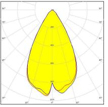
Dimensions: 280.0 mm x 35.0 mm Height: 13.42 mm ~60° beam. 8X1 variant.
