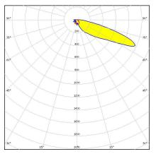
**Dimensions: 280.0 mm x 35.0 mm Height: 15.35 mm** Forward throwing beam with peak in 65°. 8X1 variant.
