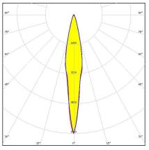
Dimensions: 280.0 mm x 35.0 mm Height: 14.51 mm ~20° beam. 8X1 variant.
