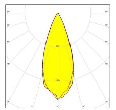
Dimensions: 280.0 mm x 35.0 mm Height: 15.00 mm ~40° beam. 8X1 variant.
