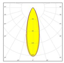
Dimensions: 9.9 mm x 9.9 mm Height: 7.50 mm ~25° diffused beam. Clip fastening
