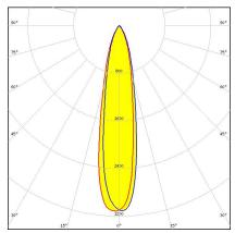
Dimensions: 9.9 mm x 9.9 mm Height: 7.50 mm ~19° real spot beam. Clip fastening for 1.6 mm thick PCB
