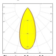
Dimensions: 9.9 mm x 9.9 mm Height: 7.50 mm ~50° wide beam. Clip fastening for 1.6 mm thick PCB
