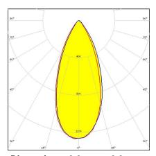
Dimensions: 9.9 mm x 9.9 mm Height: 7.50 mm ~50° wide beam. Clip fastening for 0.8 mm thick PCB
