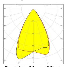
Dimensions: 9.9 mm x 9.9 mm Height: 7.50 mm ~55° wide beam and holder with
