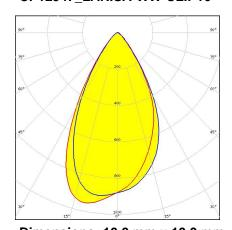
Dimensions: 10.0 mm x 10.0 mm Height: 7.50 mm ~55° wide beam. Clip fastening for 1.6 mm thick PCB
