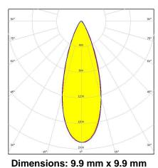
**Height: 7.50 mm**~30° medium beam. Clip fastening for 0.8 mm thick PCB.
