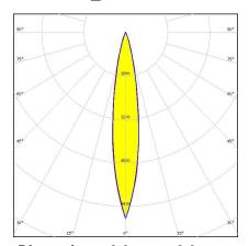
Dimensions: 9.9 mm x 9.9 mm Height: 7.50 mm ~19° spot beam and holder with location pins
