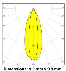
**Height: 7.50 mm** ~40° x 20° oval beam. Clip fastening for 1.6 mm thick PCB.
