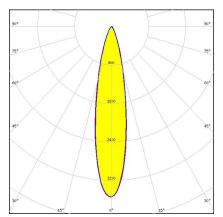
**Dimensions: 21.6 mm x 21.6 mm Height: 13.10 mm** ~13° diffused spot beam. Assembly with thinner white holder, installation tape and location pins.
