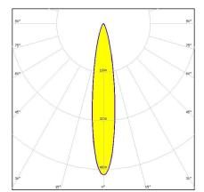
Dimensions: 21.6 mm x 21.6 mm Height: 13.10 mm ~15° diffused spot beam optimized for CREE XP-E. Assembly with
