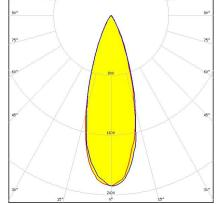
Dimensions: 21.6 mm x 21.6 mm Height: 13.10 mm ~30° medium beam optimized for
