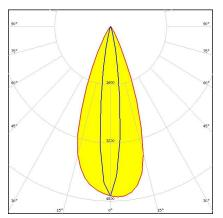
**Dimensions: 21.6 mm x 21.6 mm Height: 13.10 mm** ~40° x 13° oval beam. Assembly with thinner white holder, installation tape and location pins.
