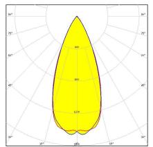
Dimensions: 21.6 mm x 21.6 mm Height: 12.90 mm ~30° medium beam optimized for Nichia 19. Assembly with black holder and installation tape.
