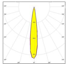
Dimensions: 21.6 mm x 21.6 mm Height: 13.10 mm ~8° spot beam. Assembly with thinner white holder, installation tape and location pins.
