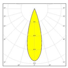
Dimensions: 21.6 mm x 21.6 mm Height: 14.80 mm ~36° wide beam. Assembly with black SC2-holder.
