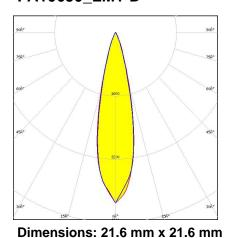
Height: 14.04 mm ~14° diffused spot beam optimized for CREE MC-E. 14.04 mm high
