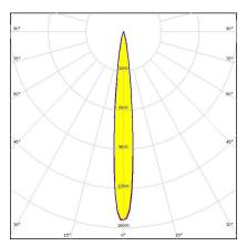
Dimensions: 21.6 mm x 21.6 mm Height: 14.80 mm ~14° diffused spot beam
