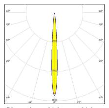
Dimensions: 21.6 mm x 21.6 mm Height: 14.70 mm ~9.6° spot beam optimized for
