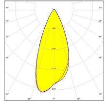
Dimensions: 21.6 mm x 21.6 mm Height: 14.70 mm ~40° wide beam optimized for CREE
