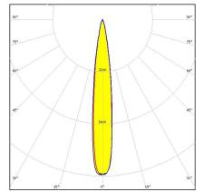
Dimensions: 21.8 mm x 21.8 mm Height: 14.70 mm ~8.5° spot beam with light, black holder.
