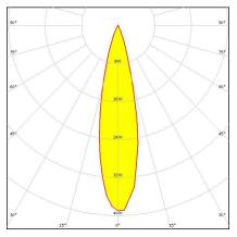
**Dimensions: 21.6 mm x 21.6 mm Height: 14.70 mm** ~25° medium beam optimized for CREE XP-E. 14.7 mm high assembly with installation tape.
