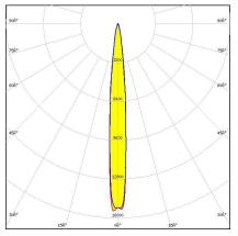
Dimensions: 21.6 mm x 21.6 mm Height: 14.70 mm ~8.5° spot beam optimized for CREE XP-E. 14.7 mm high assembly.
