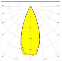
Dimensions: 21.6 mm x 21.6 mm Height: 14.70 mm ~40° wide beam optimized for CREE XP-E. 14.7 mm high assembly.
