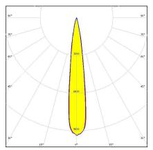
Dimensions: 21.6 mm x 21.6 mm Height: 13.50 mm ~9.6° spot beam optimized for Nichia NS6x83. 13.3 mm high assembly with installation tape.
