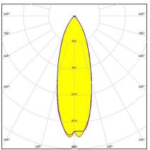
Dimensions: 21.6 mm x 21.6 mm Height: 13.90 mm ~40° wide beam optimized for Osram
