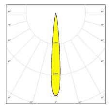
Dimensions: 21.6 mm x 21.6 mm Height: 14.70 mm ~8.5° spot beam optimized for CREE XP-E. 14.7 mm high assembly with installation tape.
