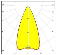
Dimensions: 21.6 mm x 21.6 mm Height: 14.30 mm ~40° wide beam optimized for LUXEON Rebel. 14.3 mm high assembly.
