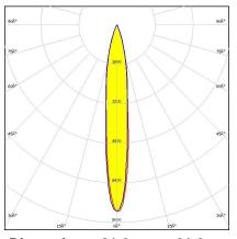
**Dimensions: 21.6 mm x 21.6 mm Height: 14.80 mm** ~9.6° spot beam optimized for CREE XM-L. 14.8 mm high assembly with installation tape.
