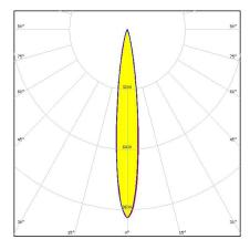
Dimensions: 21.6 mm x 21.6 mm Height: 14.70 mm ~14° diffused spot beam optimized for CREE XP-E. 14.7 mm high assembly
