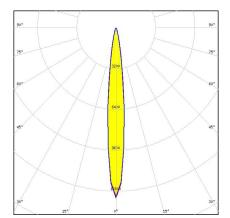
Dimensions: 21.6 mm x 21.6 mm Height: 14.30 mm ~14° diffused spot beam optimized for LUXEON Rebel. 14.3 mm high assembly.
