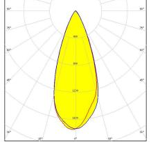
Dimensions: 21.8 mm x 21.8 mm Height: 14.70 mm ~40° wide beam with light, black holder.
