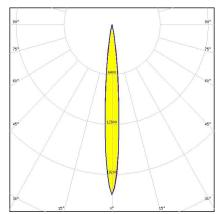
Dimensions: 21.6 mm x 21.6 mm Height: 14.30 mm ~9.6° spot beam optimized for Osram Oslon Square EC. 14.3 mm high assembly.
