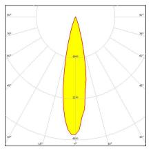
Dimensions: 21.6 mm x 21.6 mm Height: 14.60 mm ~25° medium beam optimized for CREE
