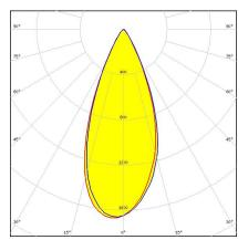
Dimensions: 21.6 mm x 21.6 mm Height: 14.50 mm ~40° wide beam optimized for LUXEON Rebel. 14.5 mm high assembly with installation tape.
