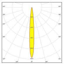
Dimensions: 21.6 mm x 21.6 mm Height: 14.70 mm ~8.5° spot beam optimized for CREE XP-E. 14.7 mm high assembly with installation tape.
