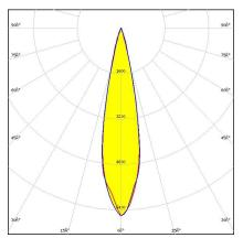
Dimensions: 21.6 mm x 21.6 mm Height: 14.04 mm ~20° spot beam optimized for CREE
