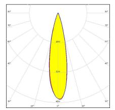
Dimensions: 21.6 mm x 21.6 mm Height: 14.80 mm ~25° medium beam optimized for LUXEON Rebel ES. 14.8 mm high assembly with installation tape.
