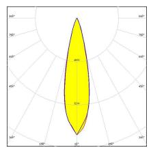
**Dimensions: 21.6 mm x 21.6 mm Height: 14.04 mm** ~14° diffused spot beam optimized for CREE MC-E. 14.04 mm high assembly with installation tape.
