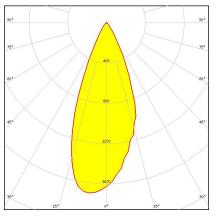
Dimensions: 21.6 mm x 21.6 mm Height: 14.60 mm ~40° wide beam optimized for CREE XB-D. 14.6 mm high assembly with installation tape.
