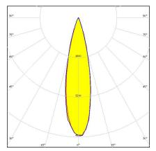
Dimensions: 21.6 mm x 21.6 mm Height: 14.30 mm ~25° medium beam optimized for Osram Oslon Square EC. 14.3 mm high assembly.
