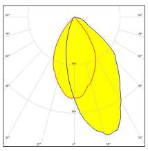
Dimensions: 111.0 mm x 111.0 mm Height: 37.00 mm Asymmetric beam for wall-washing
