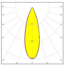
Dimensions: 50.6 mm x 50.6 mm Height: 11.90 mm ~30° medium beam with 4 optics
