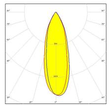
Dimensions: 50.6 mm x 50.6 mm Height: 11.90 mm ~35° medium beam with 3 optics
