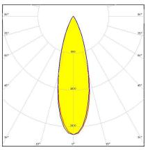
Dimensions: 50.6 mm x 50.6 mm Height: 11.90 mm ~30° medium beam optimized for Nichia NCSW219A with 4 optics
