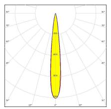
Dimensions: 50.6 mm x 50.6 mm Height: 11.90 mm ~12° spot beam with 3 optics
