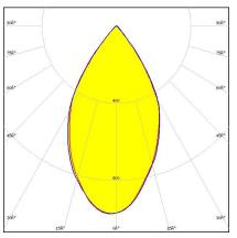
Dimensions: 49.9 mm x 49.9 mm Height: 22.58 mm ~50° wide beam compatible with LEDiL HEKLA
