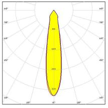
Dimensions: 49.9 mm x 49.9 mm Height: 22.58 mm ~25° wide beam. Compatible with LEDiL
