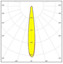
Dimensions: 49.9 mm x 49.9 mm Height: 22.58 mm ~15° spot beam. Compatible with LEDiL
