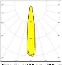
Dimensions: 49.9 mm x 49.9 mm Height: 24.00 mm ~15° spot beam
