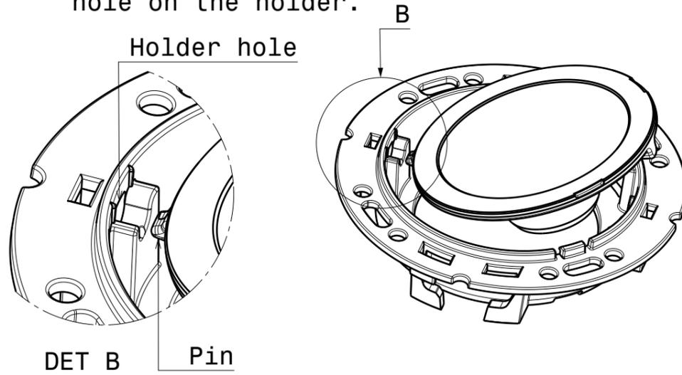
2. Press the lens under clips on the holder, ensuring both clips are fixed.
