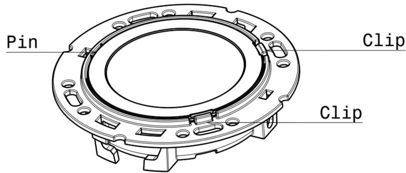
**TYPICAL CONNECTOR ASSEMBLY (including solderless BJB 47.319.2xxx 50mm as example)**
