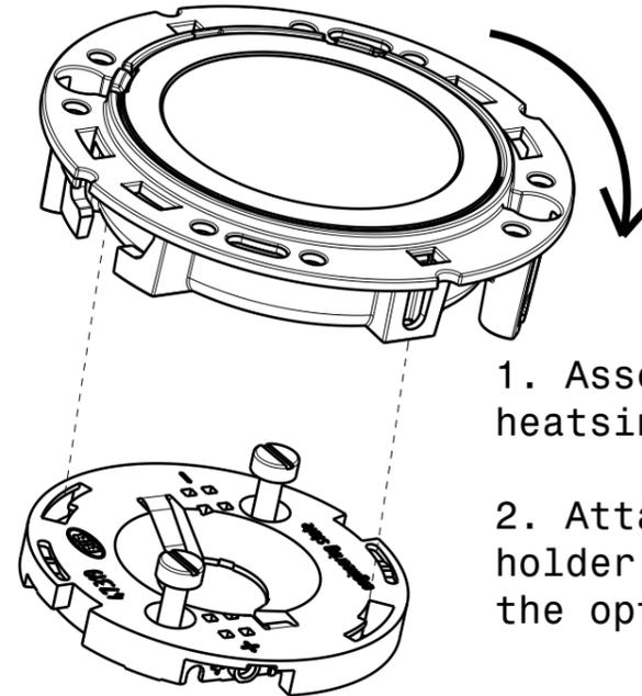
1. Assemble LED and BJB connector on heatsink with M3 screw.
