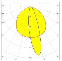
Dimensions: 119.8 mm x 19.6 mm Height: 7.60 mm Asymmetric oval beam for wall washing
