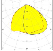
Dimensions: 119.8 mm x 19.6 mm Height: 7.00 mm Asymmetric square beam for illuminating near field shelf objects and floor/ground areas in larger environments
