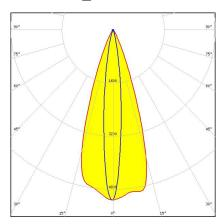
Dimensions: 26.0 mm x 26.0 mm Height: 16.20 mm ~35° + 8° oval beam. Assembly with installation tape.
