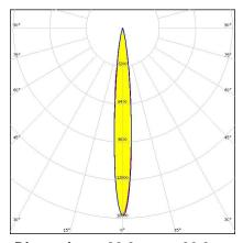
Dimensions: 26.0 mm x 26.0 mm Height: 16.70 mm ~9° smooth spot beam
