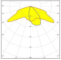
Dimensions: 119.8 mm x 25.2 mm Height: 5.60 mm Soft wide beam with good illuminance uniformity
