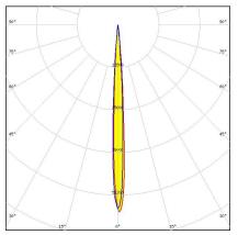
Dimensions: 37.8 mm x 37.8 mm Height: 24.00 mm ~6° real spot beam. Assembly with
