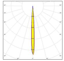
Dimensions: 37.8 mm x 37.8 mm Height: 23.88 mm ~6° real spot beam with holder
