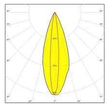
**Dimensions: 16.1 mm x 16.1 mm Height: 10.12 mm** ~35° + 15° oval beam optimized for Osram Golden Dragon+. Assembly with holder and installation tape.
