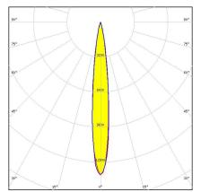
Dimensions: 16.1 mm x 16.1 mm Height: 9.66 mm ~16° diffused spot beam Assembly with holder and installation tape.
