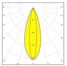
Dimensions: 16.0 mm x 16.0 mm Height: 9.50 mm ~35° + 15° oval beam. Assembly with
