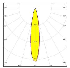
Dimensions: 16.1 mm x 16.1 mm Height: 11.00 mm ~14° spot beam optimized for Nichia NS6x83. Assembly with holder and installation tape.
