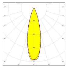
**Dimensions: 16.1 mm x 16.1 mm Height: 9.70 mm** ~30° medium beam optimized for CREE XP-E. Assembly with holder and installation tape.
