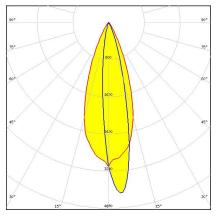
Dimensions: 16.1 mm x 16.1 mm Height: 9.70 mm Asymmetric beam for wall-washing. Assembly with black holder and installation tape.
