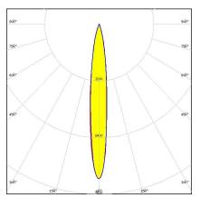
**Dimensions: 16.1 mm x 16.1 mm Height: 9.30 mm** ~14° spot beam optimized for Nichia NCSxx19. Assembly with holder, installation tape and location pins.
