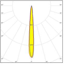
Dimensions: 16.1 mm x 16.1 mm Height: 9.50 mm ~14° spot beam optimized for Osram
