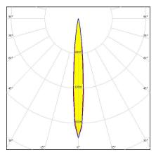
Dimensions: 50.0 mm x 50.0 mm Height: 14.50 mm ~12° smooth spot beam
