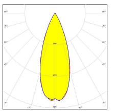
Dimensions: 50.0 mm x 50.0 mm Height: 14.50 mm ~35° medium beam
