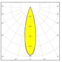
Dimensions: 50.0 mm x 50.0 mm Height: 14.50 mm ~16° medium beam
