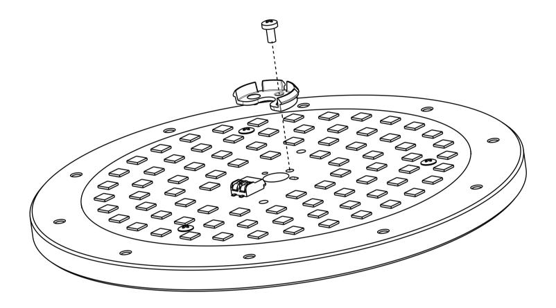
4. Fix the lens with M4 screws
