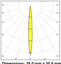
Dimensions: 35.0 mm x 35.0 mm Height: 18.00 mm ~14° spot beam
