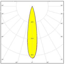
Dimensions: 35.0 mm x 35.0 mm Height: 18.00 mm ~15° spot beam
