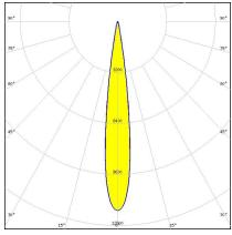
Dimensions: 35.0 mm x 35.0 mm Height: 18.00 mm ~10° spot beam
