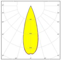
Dimensions: 35.0 mm x 35.0 mm Height: 18.00 mm ~36° spot beam
