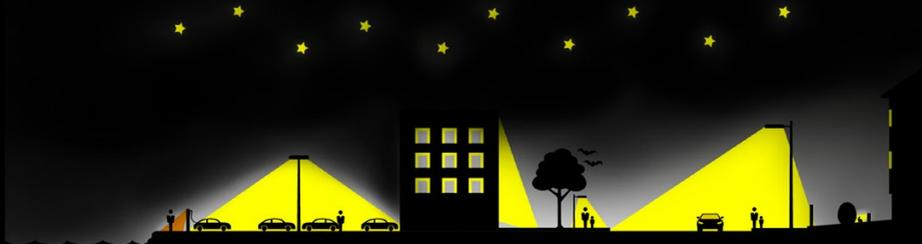
*Well designed luminaires and the right optics can reduce light pollution and skyglow.*
