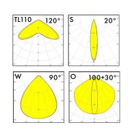
Extremely precise elliptical beam for wide coverage and reach
