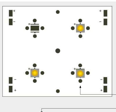
We recommend LED assembly tolerance of ±0.1 mm. For accurate positioning good solder pad design is necessary. If the solder pad is not the right size and shape the LED alignment may suffer significantly.
